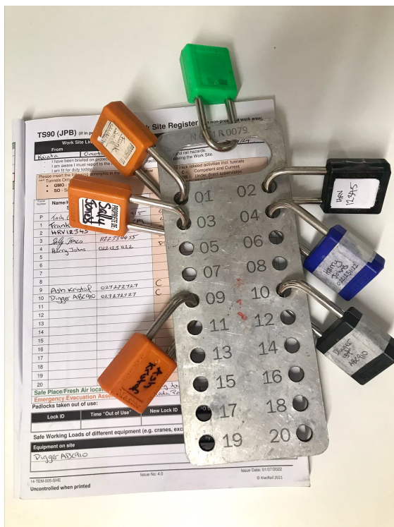
Lock On Frame and Lock on Board (Worksite Register Board)
