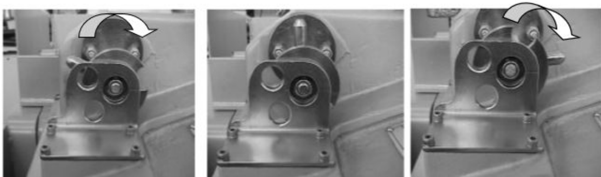
Picture showing Hand-Throw Operation
