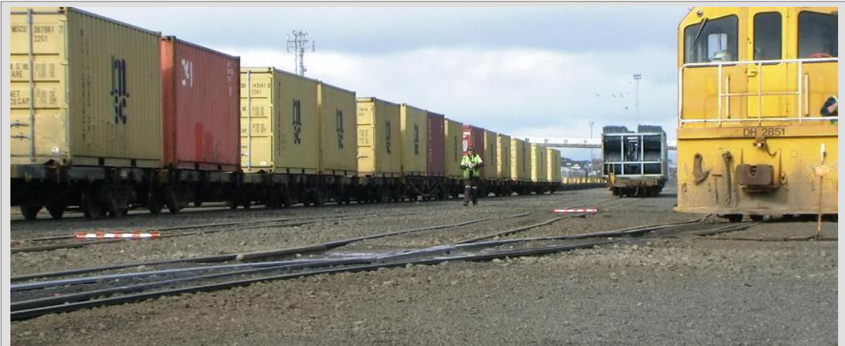
Fouling Point Marker
