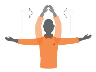
Apply Brakes for Air Brake Test
