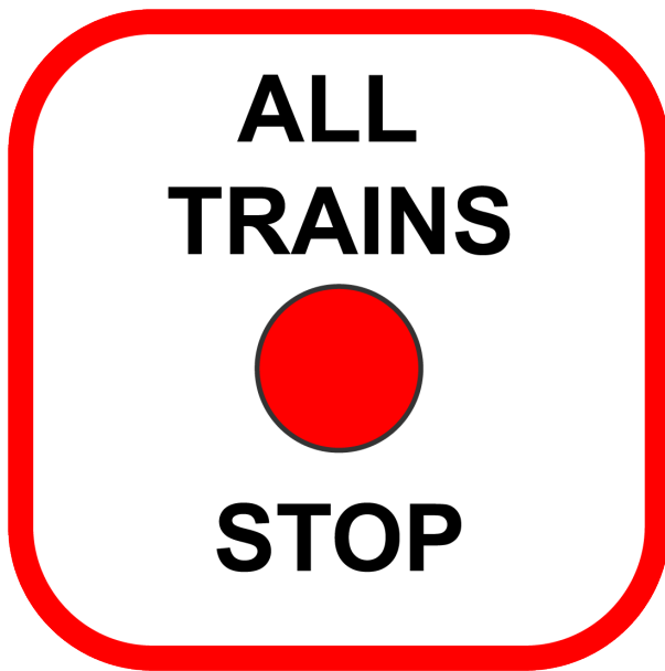
All Trains Stop Board
