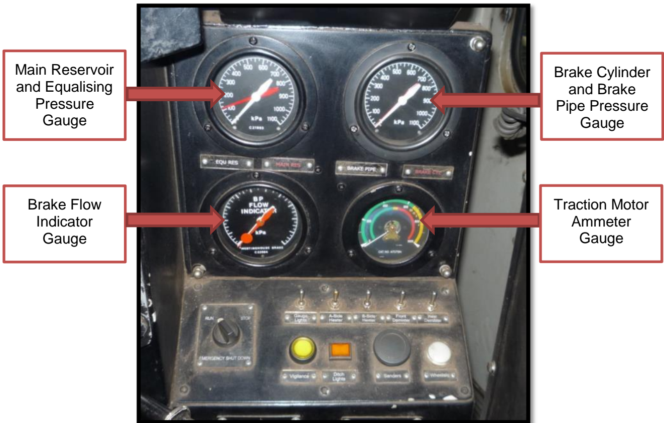
Figure 12: Control Stand Gauges
