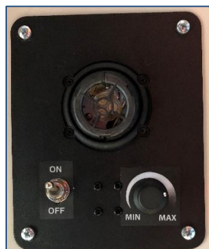
Fig. 28 Dimmer control for cab spotlights
