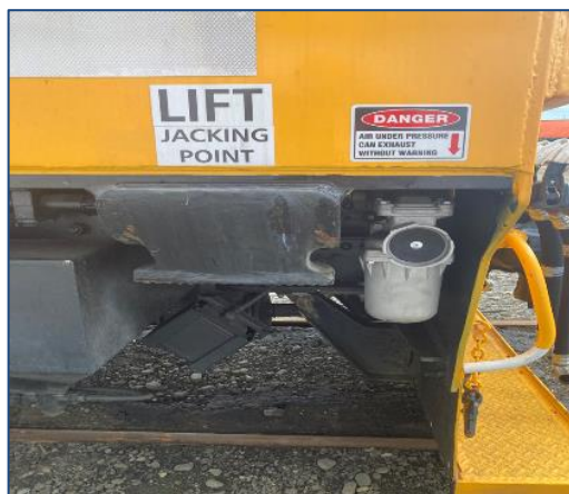
Fig. 68 KM2 vent valve warning notice
