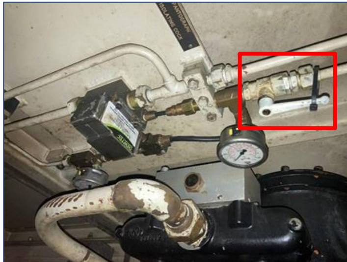
Fig. 18 Pantograph auto drop override cut out valve.
