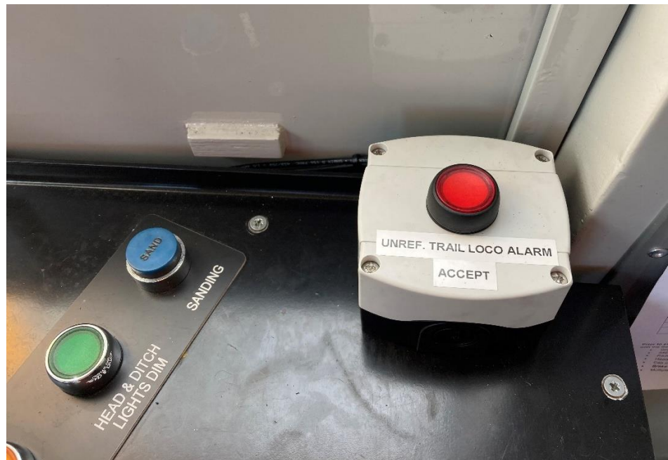
Fig. 72 Unref. Trail Loco Alarm Accept button.
