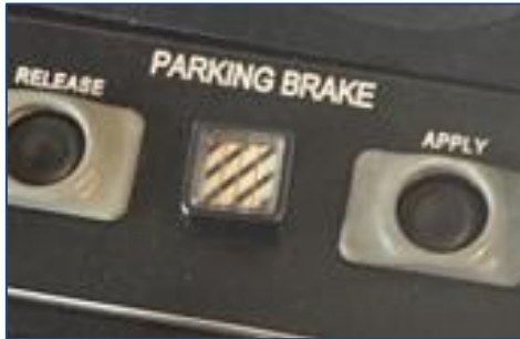
Fig. 52 Cab Park Brake controls
