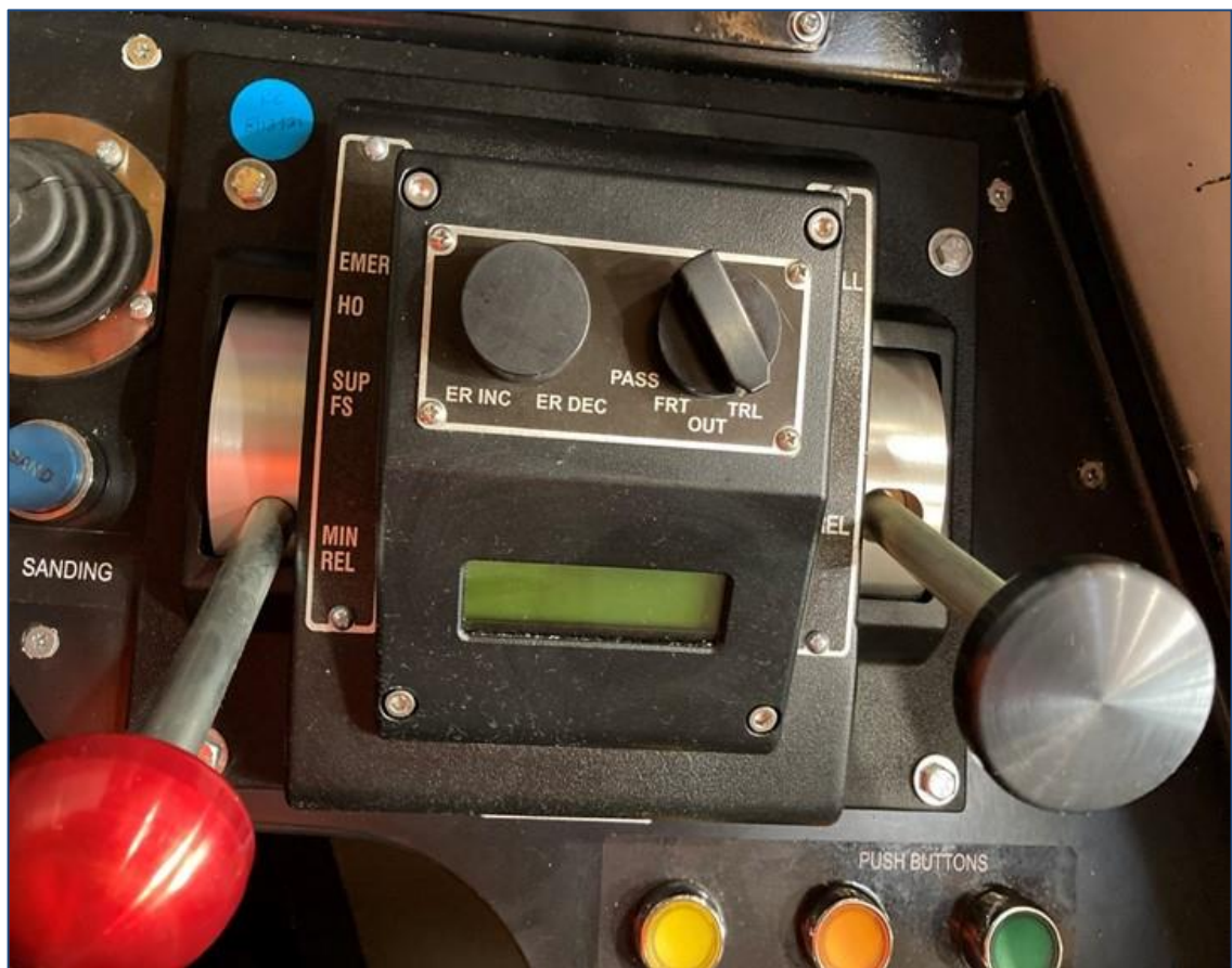
Fig. 47 Automatic (left) and Independent (right) brake handles.
