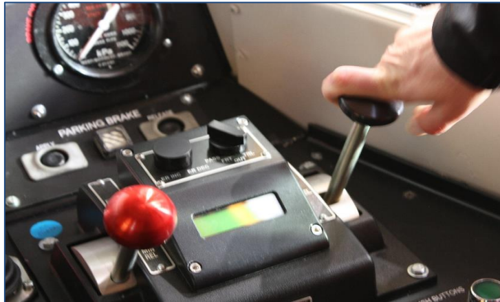
Fig. 48 Independent release - IBH pushed to the right.
