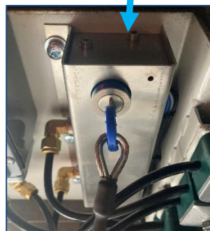
Fig. 55 Key switches to check before start up
