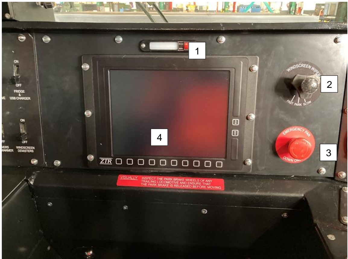
Fig. 22 Integrated Locomotive Display, Emergency Pan down button.
