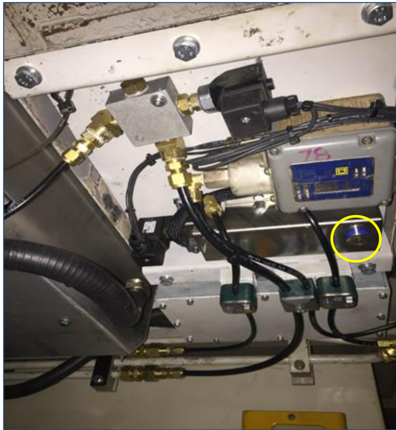
Fig. 19 Blue key used to lower Pantograph manually
