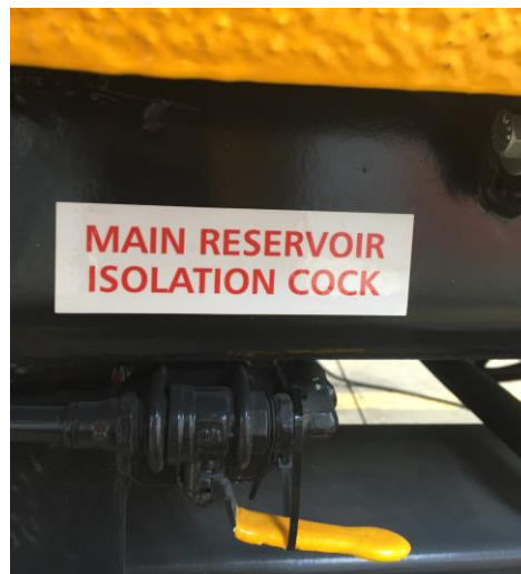
Figure 36: AKS Main Reservoir Drain Prevention Cock under B2 door
