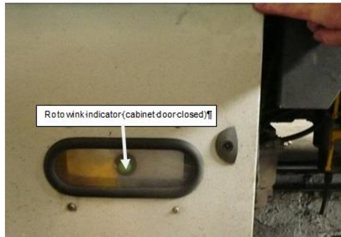
Figure 22: Park brake Rotowink indicator viewed through closed cabinet.
