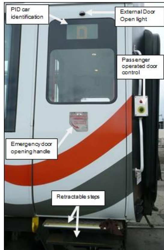
Figure 9: External view of plug door and controls.
