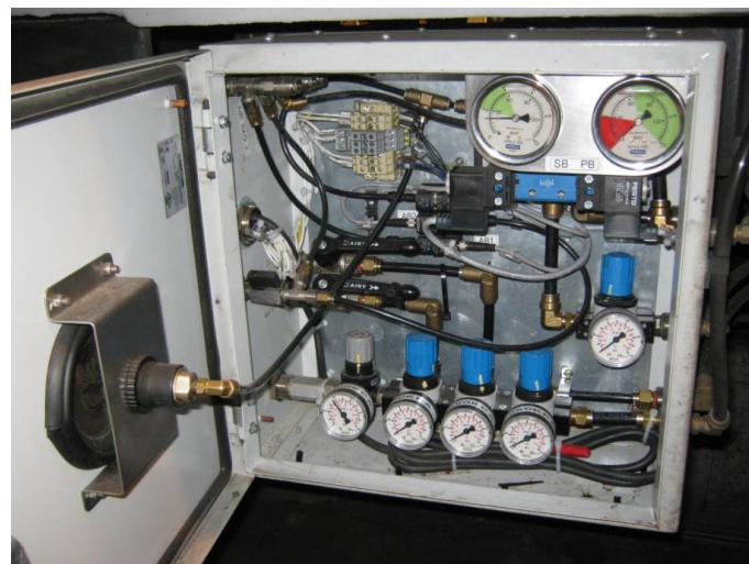
Figure 23: Park brake Rotowink indicator, Air Services Box (open).
