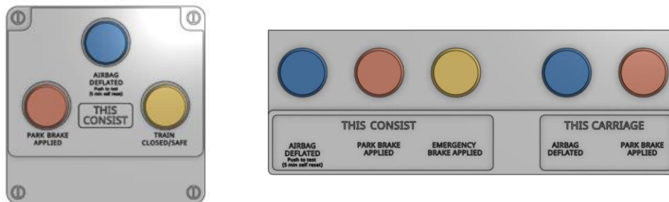
Figure 48: Train Status Panels located in AKC (left) and AKS (right).
