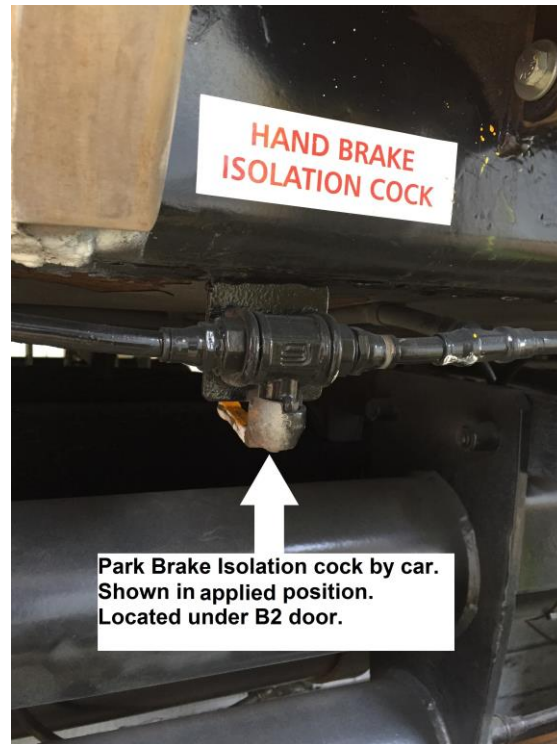
Figure 27: AKS Park Brake air isolation cock by car.
