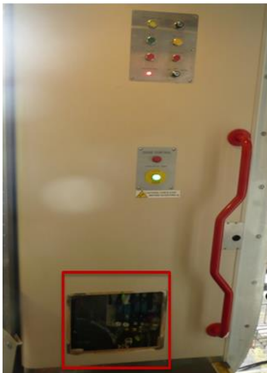
Figure 30: Location of access panel for door and step isolation cocks.
