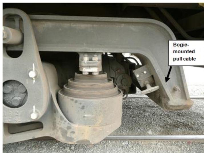
Figure 24: P11 Bogie location of park brake mechanical release handle.
